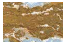
Galvanised Steel 20 µm after 6 weeks
